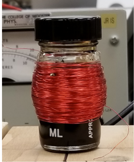
FIG. 1: The ferrofluid electromagnetic generator constructed. Inside the bottle is 15 ml of ferrofluid. Around the outside is 500 turns of magnet wire.
