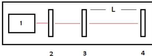
FIG. 4: A schematic of the optical channel. Object 1 is the light source. A broad single slit, component 2, makes a focused beam to pass to 3. Component 3 is a double slit with slit width  $a = 0.085$  mm and separation distance  $d = 0.343$  mm. A screen was used to block one slit when needed. Lastly, 4 is the intensity measurement device at  $L = 0.5$  m from 3.
