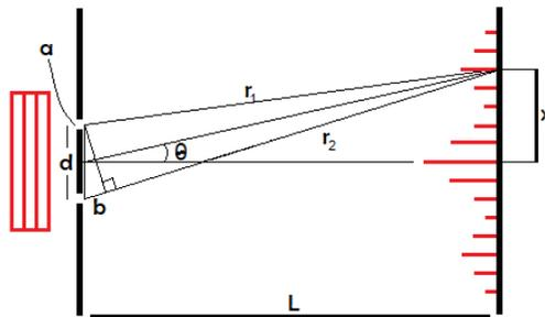
FIG. 2: A plane wave incident on a double slit with separation distance  $d$  and slit width  $a$ . The observation screen is a distance  $L$  from the double slit, while points of interest on it are a distance  $\pm x$  from the central maximum
