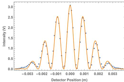
FIG. 6: The double slit data for the laser diode plotted with the theoretical double slit interference prediction, using  $\lambda_l = 640$  nm and  $I_{max} = 3.06$  V.
