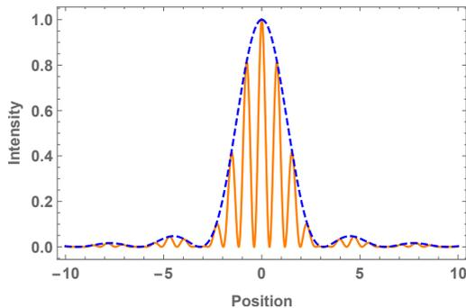
FIG. 3: Predicted intensity patterns for single slit diffraction (dashed) and double slit interference (solid).
