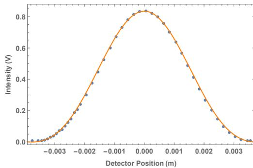
FIG. 5: The single slit data for the laser diode plotted with the theoretical single slit diffraction prediction, using  $\lambda_l = 640$  nm and  $I_{max} = 0.835$  V.
