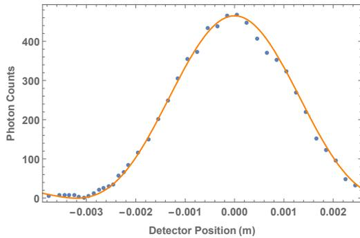
FIG. 7: The single photon single slit data plotted alongside the theoretical single slit diffraction pattern using  $\lambda_p = 545$  nm, and  $I_{max} = 468$  counts.
