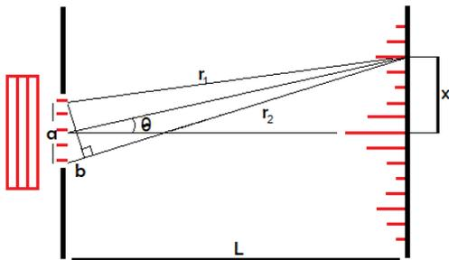
FIG. 1: A plane wave incident on single slit with width  $a$ . The observation screen is a distance  $L$  from slit, while points of interest on it are a distance  $\pm x$  from the central maximum.
