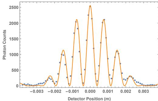
FIG. 8: The single photon double slit data plotted alongside the theoretical double slit interference, using  $\lambda_p = 545$  nm, and  $I_{max} = 2560$  counts.
