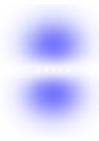
FIG. 3: A density plot describing the HG_{01} , first order Hermite Gaussian 'even' mode
