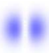
FIG. 4: A density plot describing the HG_{10} , first order Hermite Gaussian 'odd' mode
