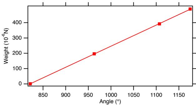
FIG. 6: The weight versus the torsion angle. The slope gives us the torsion constant  $K_{tor} = (137 \pm 208) \times 10^{-6}$  N/deg.
