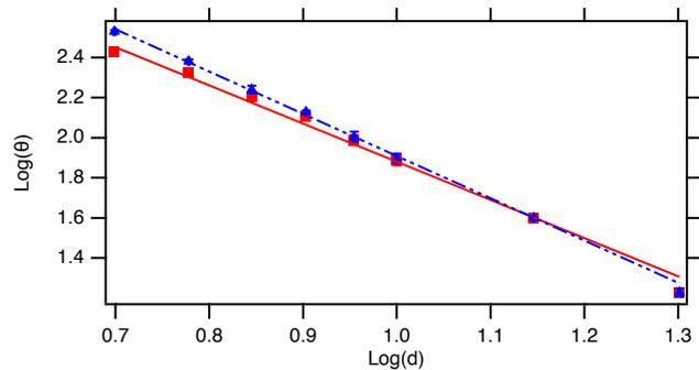
FIG. 4: The logarithm of the angle versus the logarithm of the distance with the corrected angle in blue triangles and a dashed line and the original angle in red squares. The slope of these lines is equal to the exponent  $n$  in the equation  $F \propto 1/d^n$ . For the corrected angle  $n = -2.107 \pm 0.018$  and for the original angle  $n = -1.905 \pm 0.017$ . which are both within 5% of the accepted value of 2.
