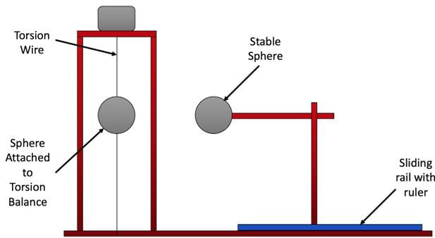
FIG. 1: Apparatus used to investigate the relationship between force and charge or force and distance.
