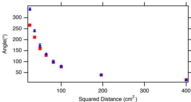
FIG. 3: The angle measured versus the distance squared with the corrected angle is in blue triangles and the original angle is in red squares. This shows the relationship between force and distance is  $F \propto 1/d^2$ .
