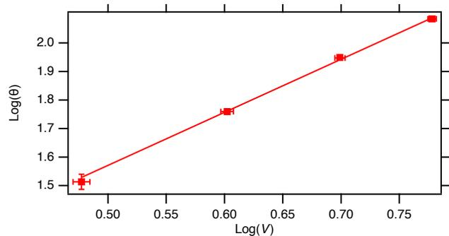
FIG. 5: The logarithm of the force measured as an angle versus the logarithm of the voltage applied to the spheres. The slope  $n$  is the exponent for  $q^n$  and is  $1.86 \pm 0.08$  which is within 7% of the accepted value of 2. This shows the relationship between force and charge to be  $F \propto q^2$  with  $q = q_1 = q_2$ .
