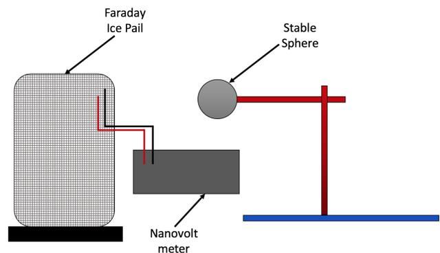
FIG. 2: Apparatus used to measure the charge on the sphere.
