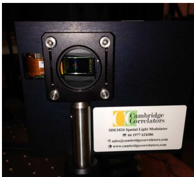
FIG. 5: The SDE1024 has a twisted nematic mode liquid crystal display screen in which the laser beam is directed at. The display screen visually produces the hologram needed to produce the LG modes.
