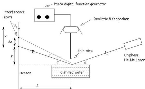
**Fig.1. The schematic of the apparatus.**
